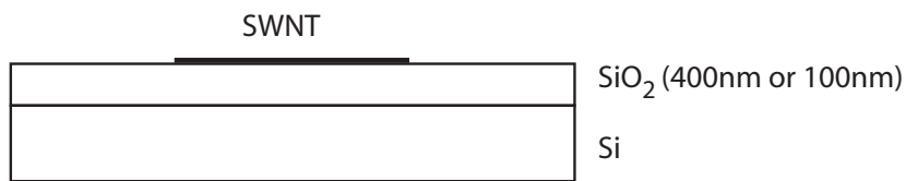
Figure 3.2: At 1000^\circ Celsius, carbon atoms from methane gas stick to the surface of the wafer, growing into nanotubes.
