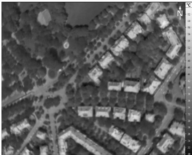
Fig. 1. False-colour thermal image taken on 16 July 2004, c. 12:00 CET. The image shows an intersection in the city of Basel at an air temperature of c. 25 °C. Temperatures range from around 22 °C (shaded tree crowns) to c. 40 °C (asphalted streets) and up to 50 °C (roofs).
